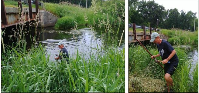
Sally Schultz installing a thermistor (continuous read thermometer) into Door Creek
